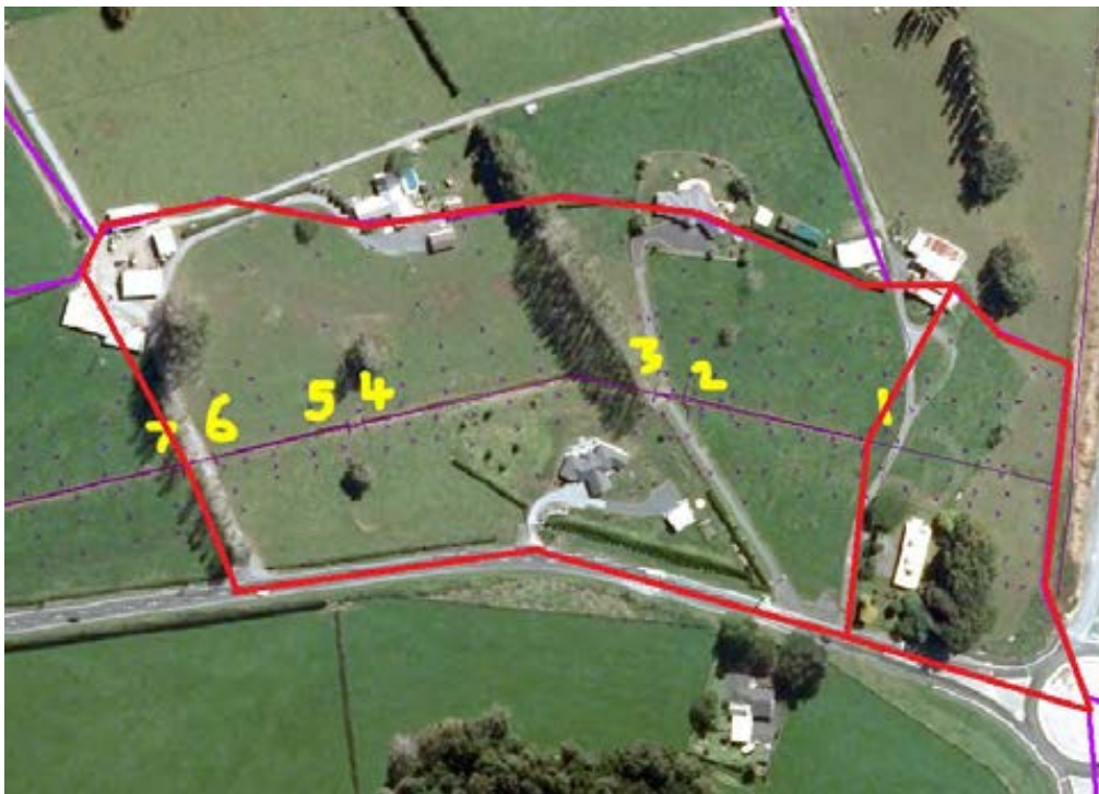
Figure 7: Catchment area (outlined in red) and location of surveyed cross-sections for Te Otamanui upper catchment
