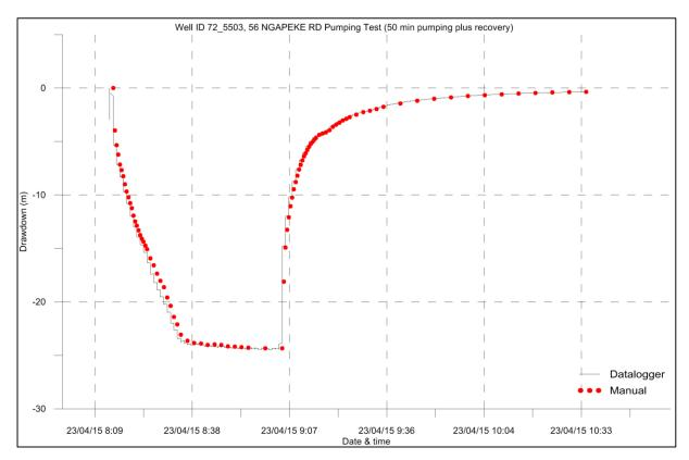
Figure A 3.11 Drawdown and recovery plot for well 72\_5503.
