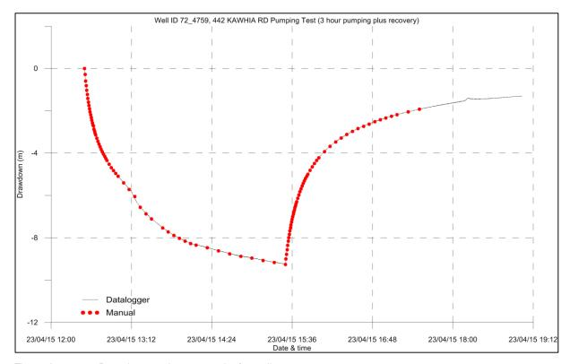
Figure A 3.13 Drawdown and recovery plot for well 72\_4759.
